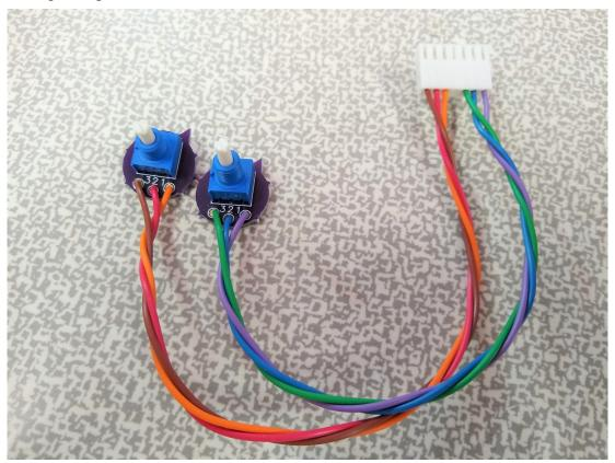
Insert the little terminals into this block as shown in the chart below.
