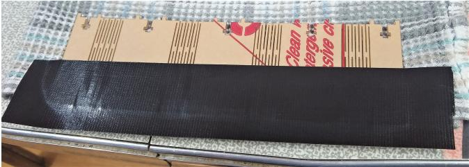
Start peeling up the tape at one corner of the paper. It should lift the paper off the plastic. If not, give it some help with your fingernail. Slowly lift the tape, being sure that it's taking the paper with it. Peel the rest of the paper off the piece, section by section.
