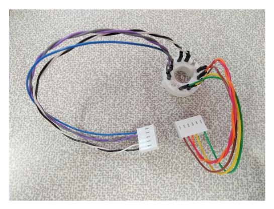
Slide one piece of heat-shrink tubing over each wire on the CRT socket, making sure that each piece is seated against the socket. Shrink all the tubing pieces onto the CRT socket terminals using a match or lighter for heat, or a heat gun if you have one. It is best to hold the socket assembly by the wires when doing this, so that you don't burn your fingers. Don't worry, the heat shrink tubing is flameproof.
