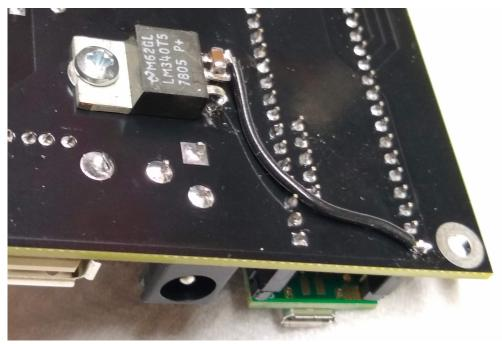
28) Strip 1/8" of insulation from each end of the black wire. Solder one end to pin 3 of the 7805, the end leg with the capacitor. Solder the other end to pin 48 of U2, the Teensy pin nearest the corner of the board.
