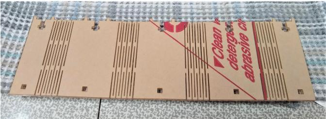
Tear off a piece of duct tape a bit longer than the piece. Press the tape onto the edge of the piece so that it hangs over the edge by about half an inch. Rub firmly on the tape along the edge of the plastic piece to make it stick well. Be sure to stick it to every slot, so they will all be pulled up.
