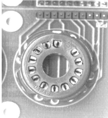
Solder each socket at two opposite pins first. Press the socket against the board while reheating these two pins one at a time to be sure the socket is fully seated. Then solder the other pins.
