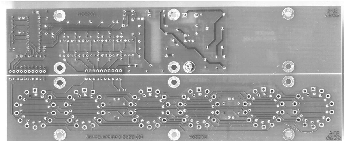
Bottom of NC620A PC Board (before separating)
